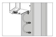
Protective bonding circuit – Double point connection
