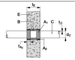
Application in a rigid wall (with Hilti Firestop Acrylic Sealant CFS-S ACR - A<sub>2</sub>)
