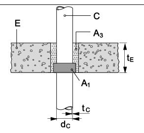
Application in a rigid floor (with cementitious mortar - A<sub>3</sub>)
