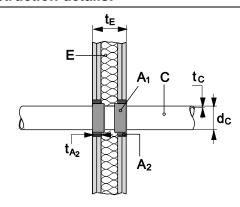
Application in a flexible wall (with Hilti Firestop Acrylic Sealant CFS-S ACR - A<sub>2</sub>)
