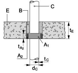
Application in a rigid floor (with Hilti Firestop Acrylic Sealant CFS-S ACR - A2)
