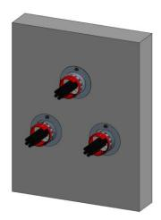
Zero distance (horizontal/vertical distance between flanges linear or cluster)
