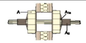
Figure 5: Filler (A<sub>1a</sub>) plus 2 layers of putty (A<sub>2</sub>)
