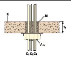
Figure 6: Mortar as gap filler (M)
