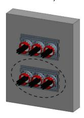
Zero Distance between Devices - For Double Gangplate installation:
