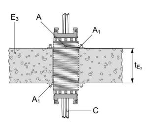
Section – CFS-SL GA M/L in Timber Walls and Floors
