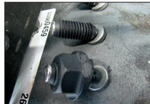
Bent X-BT-MF in internal test
