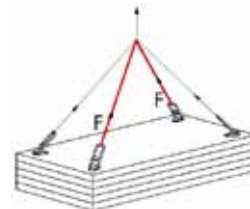
Fig. 5: statically indeterminate suspension gear
