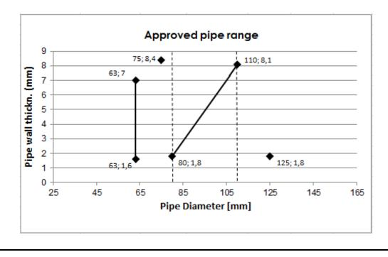
2.2.4 PVC pipes acc. to EN 1452-2, EN 1329-1, EN 1453-1
