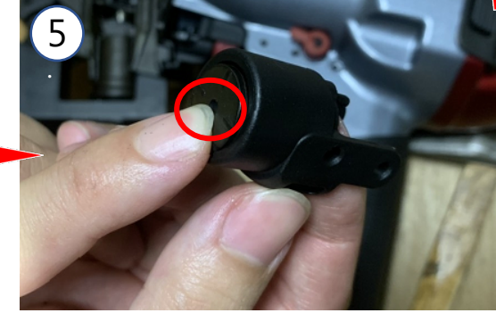
5,6&7. Hold down the contact arm with index finger to prevent parts from falling out and insert arm guide in the direction shown hereunder
