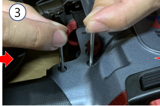
5,6&7. Hold down the contact arm with index finger to prevent parts from falling out and insert arm guide in the direction shown hereunder
