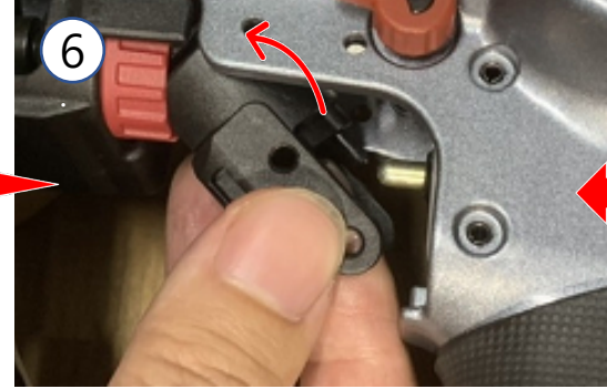
5,6&7. Hold down the contact arm with index finger to prevent parts from falling out and insert arm guide in the direction shown hereunder
