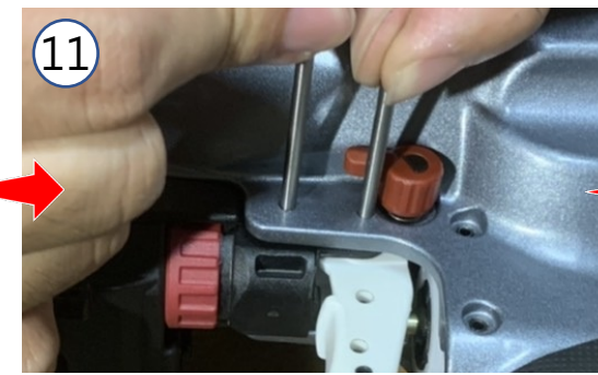
11&12. Use rod (Ø2.8) to stabilize the arm guide and trigger, then insert roll pin(100966)
