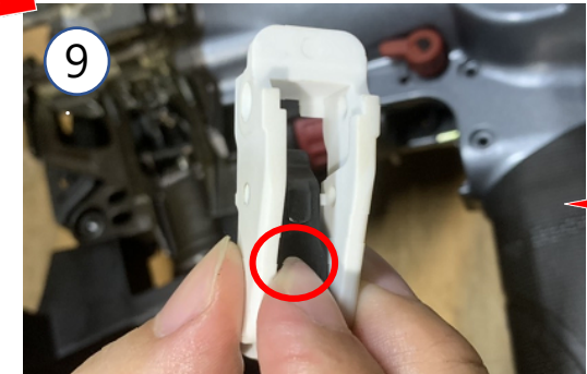
9. Place index finger on trigger rocker
