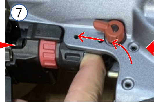
5,6&7. Hold down the contact arm with index finger to prevent parts from falling out and insert arm guide in the direction shown hereunder
