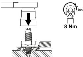
The tightening torque is **8 Nm**. Exceeding or falling below this tightening torque value is not allowed. Tighten the nut using torque tool X-BT 1/4" (8 Nm), torque wrench or Hilti screw driver SBT 4-A22, SFC 18-A, SFC 22-A (torque setting 5) with socket S-NS.
