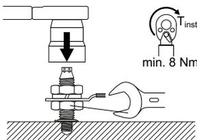
Hold the bottom nut with a spanner while tightening the upper nut.
