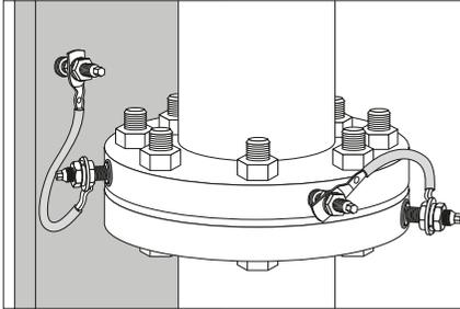
Functional and protective bonding of pipes <sup>\*)</sup>
