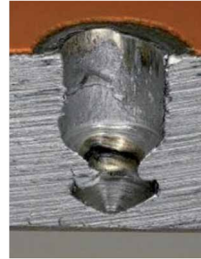
Steel base material after 10 years of exposure to sea water and pull-out of the X-BT fastener. The hole appears clean and no evidence of corrosion is visible.
