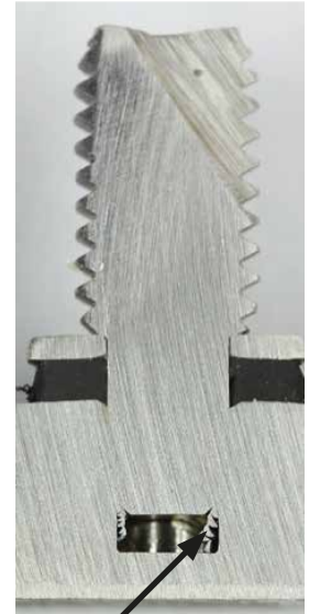
Displaced base material
