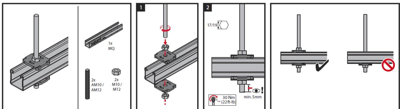
Hilti drilled plate MQZ-L11 and Hilti drilled plate MQZ-L13
