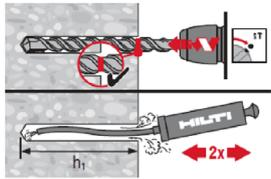
Cleaning needed in downward and horizontal installation direction with drill hole depth.
