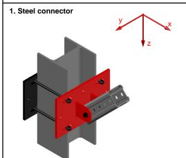
The values for Mx, My and Mz take into account the eccentricity between load application at hexagonal bolt axis and baseplate.
