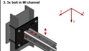
3rd bolt is just an option to standard 2 bolt solution. The 3rd bolt is not a part of standard package and has to be ordered separately. It has to be placed in the direction of the main load (this case vertically) as pictured in the next hole of connector and MI System girder connected to it.
