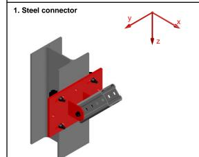
The values for Mx, My and Mz take into account the eccentricity between load application at hexagonal bolt axis and baseplate.
