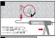
For overhead installation and installation with embedment depth  $h_{\text{ef}} > 250$ mm the injection is only possible with the aid of extensions and piston plugs.
