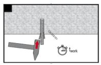
For overhead installation use piston plugs and fix embedded parts with e.g. wedges.
