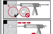
Inject the adhesive starting at the back of the hole, slowly withdrawing the mixer with each trigger pull.
