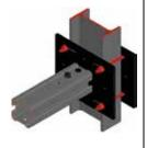
Connector used for fixing MIQ girder, perpendicularly to flange (width of 165-235mm) of structural steel open section, perpendicularly to structural steel beam
