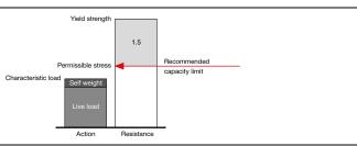
Shown load values are characteristic values. The partial safety factor for the actions is 1.5
