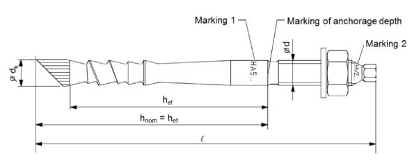
HAS-(E-)TZ / HAS-(E-)RTZ / HAS-(E-)HCR-TZ Marking 1: anchor type
