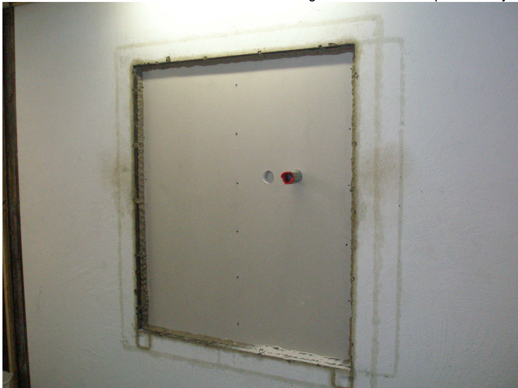
Fig. 1 Metal stud wall installed in window test rig, with opening for two 2" cable penetration assemblies, prepared by ift Centre for Acoustics
