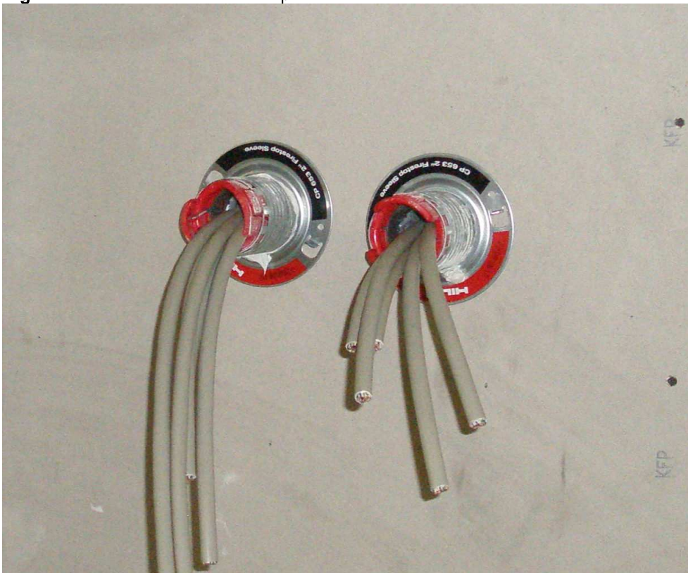
Fig. 3 2" cable penetration assembly with 5 cable pieces each
