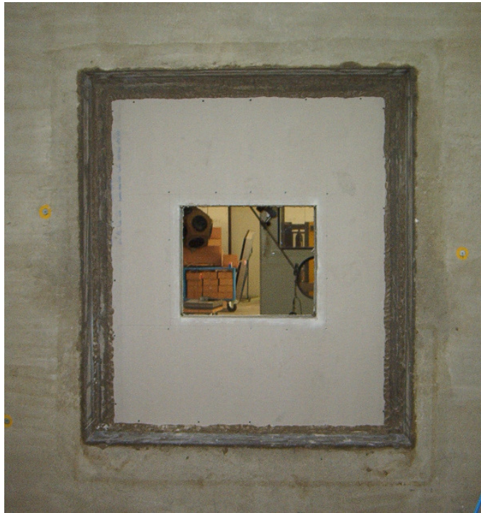
Fig. 2 Photo of metal stud partition with opening, taken by ift Centre for Acoustics – horizontal section of stud partition.
