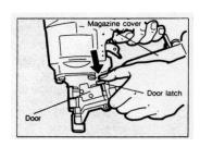
**Open the magazine:** Pull down door latch and swing door
