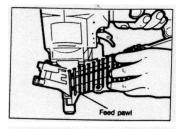
**Nail loading:** Place a coil of nails over the post in the
