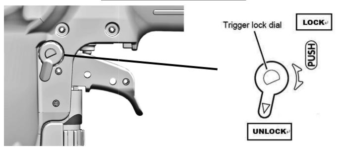
The tool is equipped with a Trigger Lock mechanism. Push and rotate the Trigger Lock Dial to the trigger free position before driving nails.
