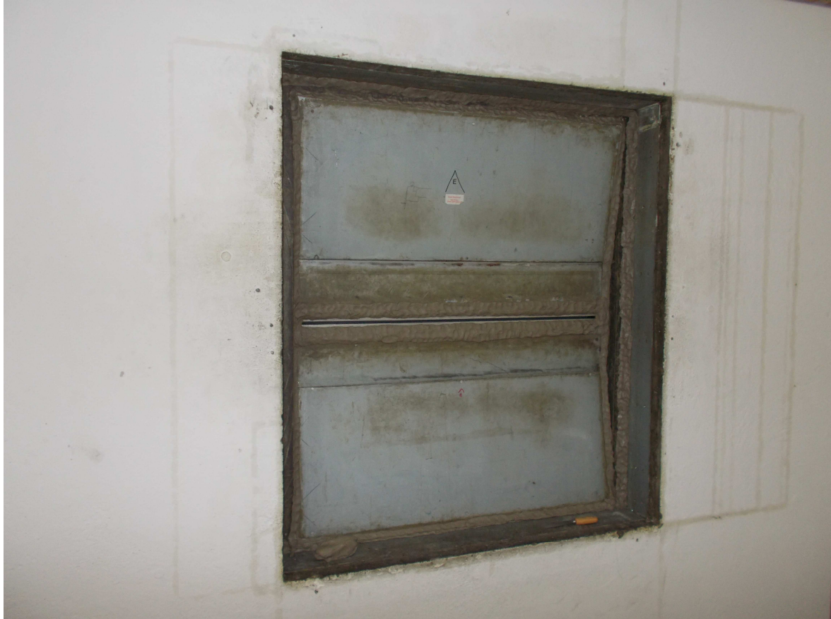
fig 4 Photo(s) of the mounted element, taken by ift Laboratory for Building Acoustics, before sealing with acrylate - sealant
