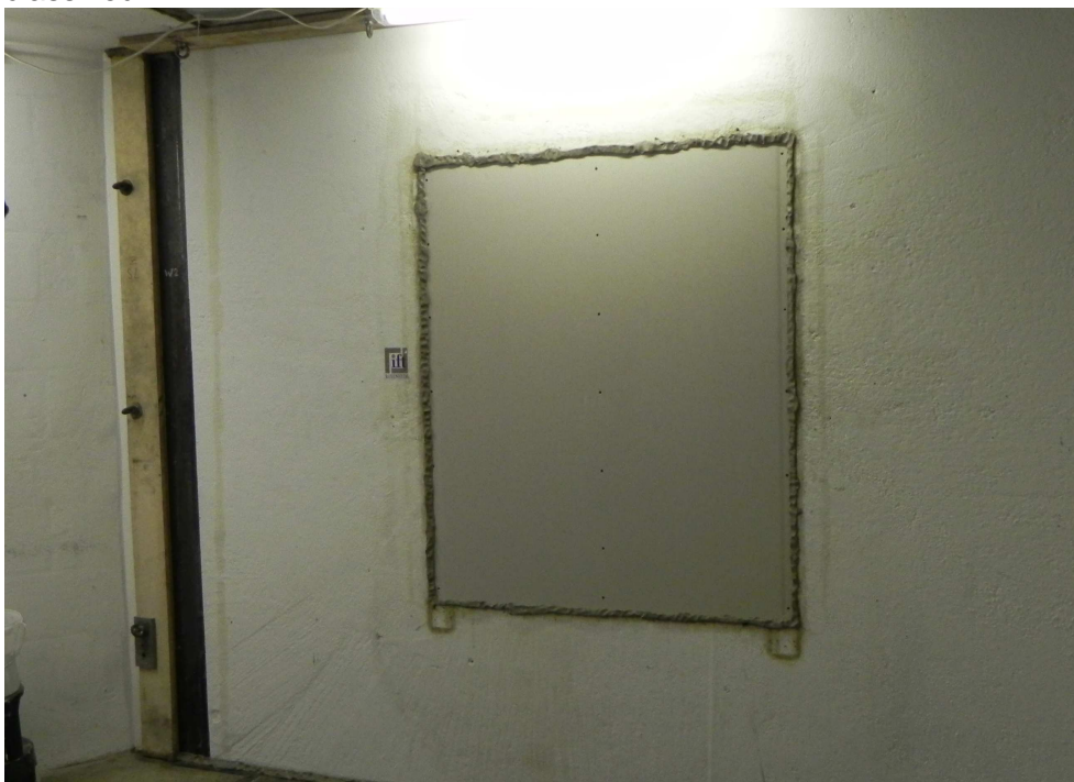
fig 1 Photos of mounted metal stud partition in test rig, taken by ift Laboratory for Building Acoustics
