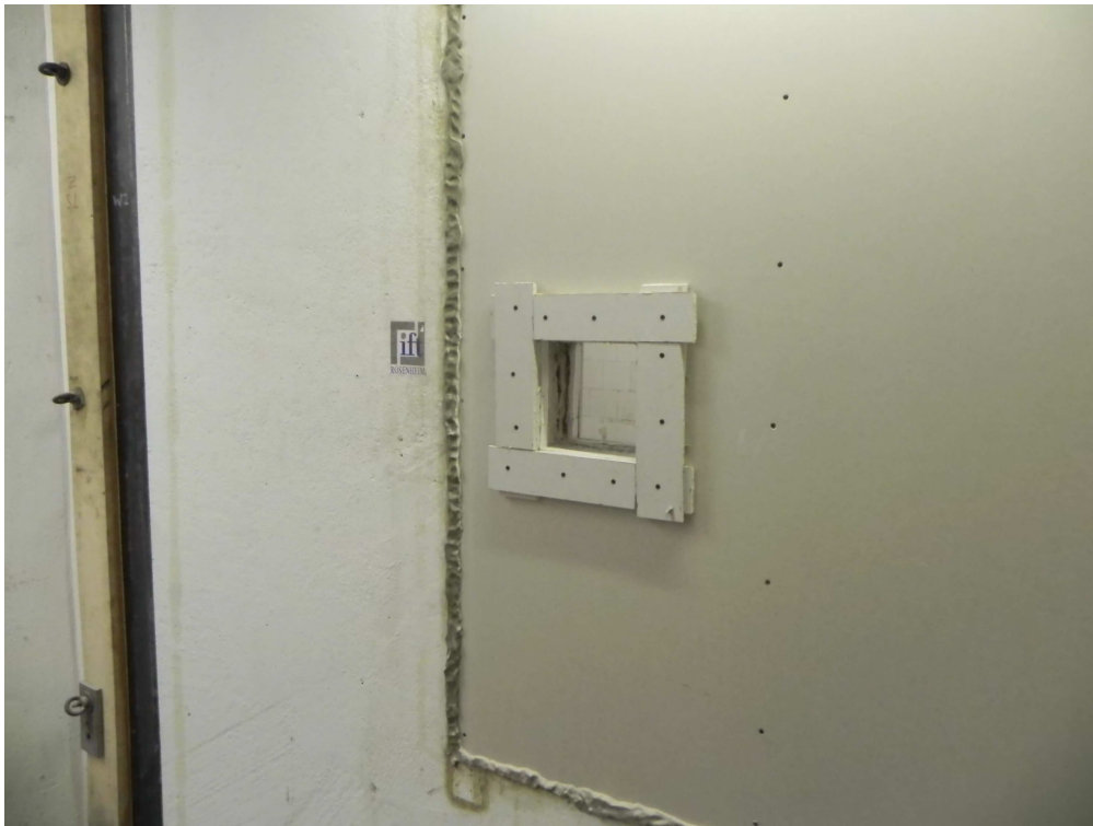
fig 2 Photos of mounted metal stud partition in the wall opening
