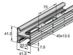
Medium-duty serrated double-channel for productive fixation of installation systems and secondary structures
