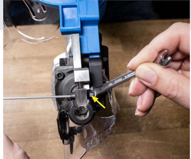
Attach the nut and pull the connection tight.
