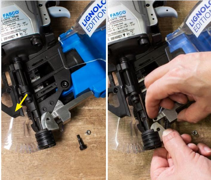
Open the door. Disassemble the pivot pin.
