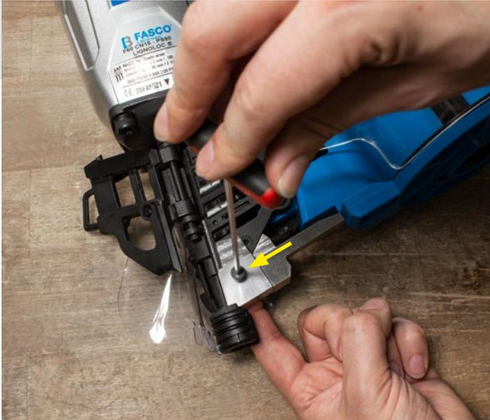
Position the front inlay and adjust the pivot pin (included in this KIT).
